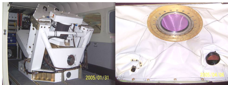
Fig. 3. View of the ANGEL Service sensor payload integrated into a Cessna 208B aircraft (left). View of the optical port on the underside of the aircraft shows the optics for the three sensors (right) with DIAL Sensor Window, 4K x 4K Digital Camera, and 1K x 1K video camera (clockwise).
