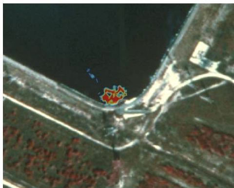
Fig. 9. ANGEL Service detection of gasoline vapor release over water at Corpus Christi, TX, with DOQQ imagery used as contextual backdrop.
