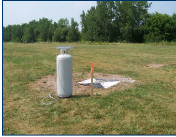
Fig. 13. Spencerport propane gas release setup that includes a compressed propane gas cylinder in the foreground connected to a flowmeter by Tygon tubing. Aerial photography target (iron cross) was used to simplify identification of the leak point.
